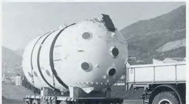
For the specialized machining of the mechanical flange connecting the dual pressure hull sections, the aft pressure hull section was transported some 35 miles to another facility.
