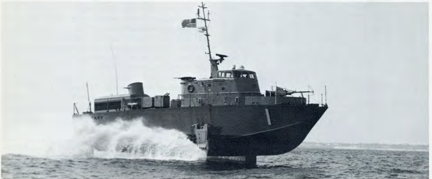
The Grumman hydrofoil gunboat "Flagstaff" (PGH-1) flies above the waves during a trial run off the coast of Palm Beach, Fla. The vehicle, built for the U. S. Navy, utilizes the Grumman base at West Palm Beach where PX-15 will be berthed.
