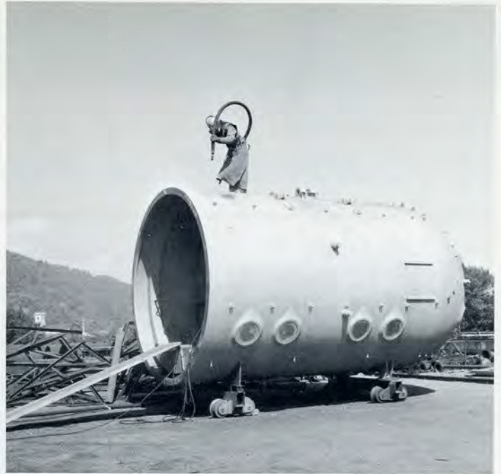
Poised like an intruder from outer space, a workman sand-blasts the PX-15 pressure hull following heat treatment. Epoxy and final paint were then applied to the vehicle.
