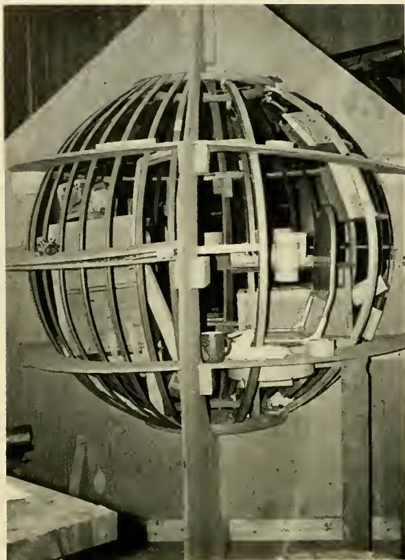
Fig. 9 28 Mockup for second JOHNSON SEA LINK acrylic sphere.
