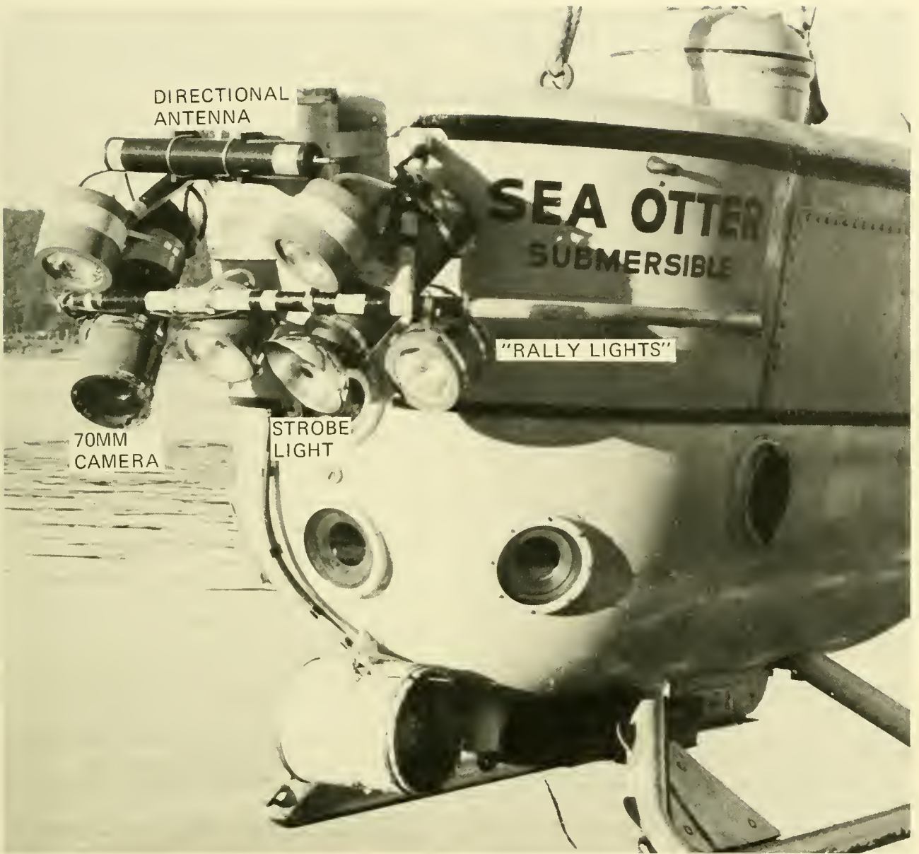
Fig. 10.3 Viewing lights, camera and strobe light, and homing antennae clustered on the brow of SEA OTTER. (Arctic Marine)
