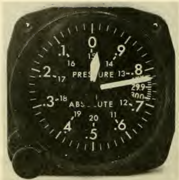
Fig 9 17 Cabin pressure indicator (Altimeter). (Mr. A. P. Ianuzzi, Naval Facilities Eng. Comm.)
