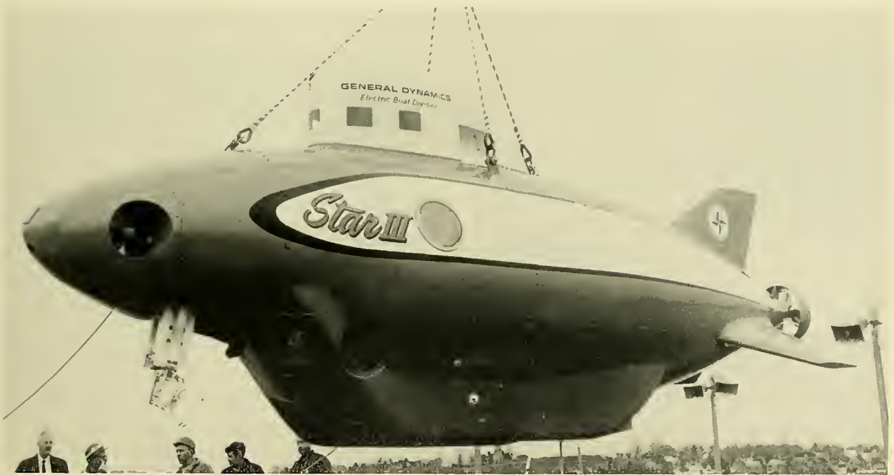
Fig. 8.16 STAR III and BEAVER . Showing two different configurations of fixed stem stabilizers. (Gen. Dyn. and North American Rockwell)
