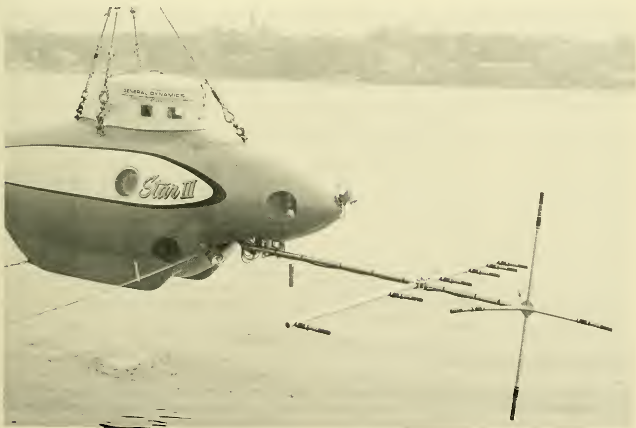
Fig. 11.2 Acoustic receiving array on STAR III . (USNUSL)
