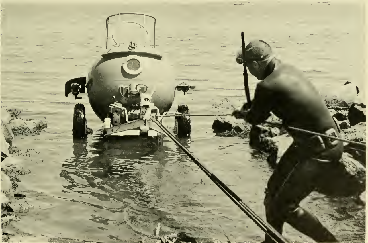
Fig 12.4 The 1 \frac{1}{4} -ton STAR I presents fewer handling problems than its large counterparts. (Gen. Dyn. Corp.)
