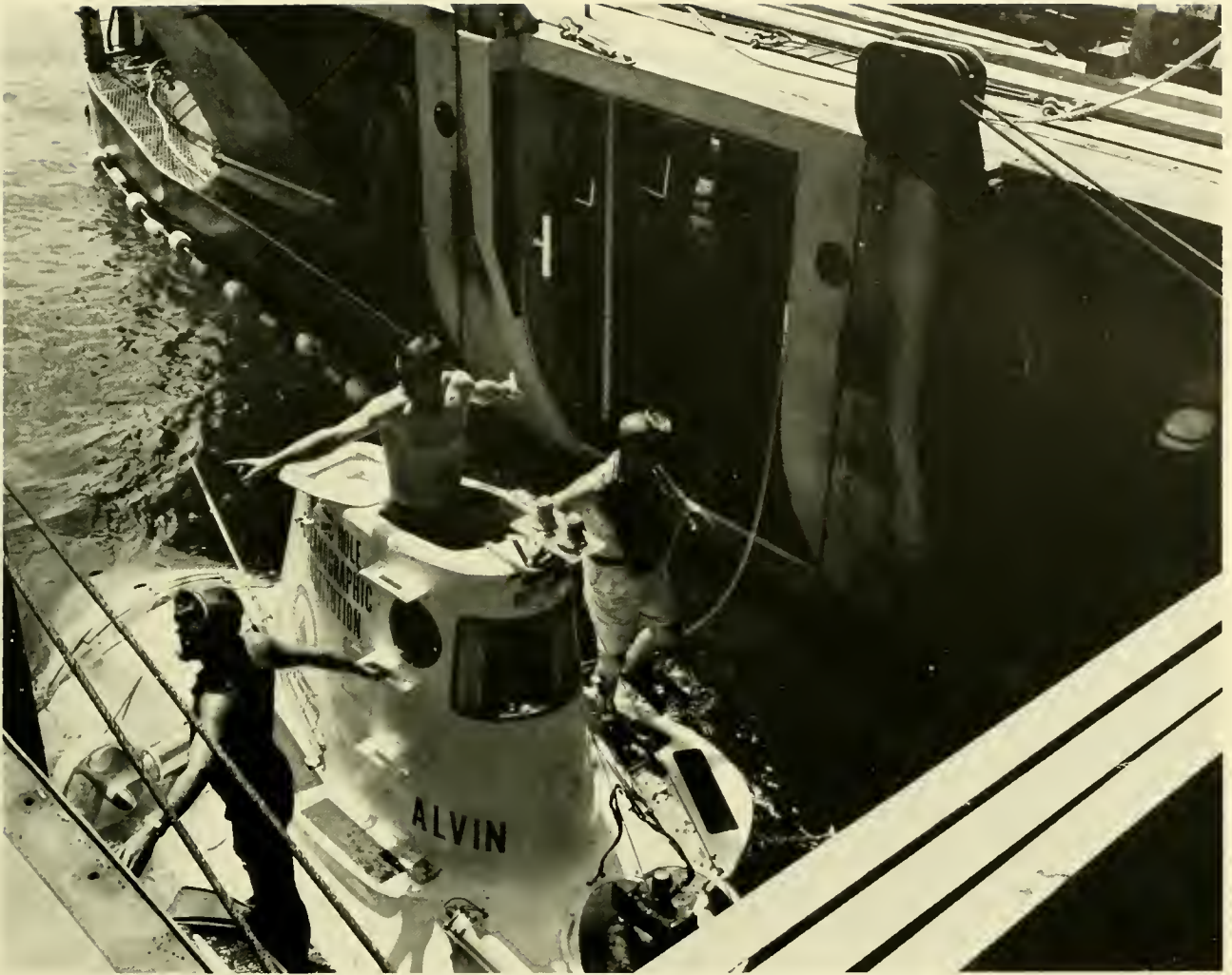
Fig. 13.4 In moderate seas the close quarters between LULU's pontoons make line-handling and control of ALVIN an exacting task. (NAVOCEANO)
