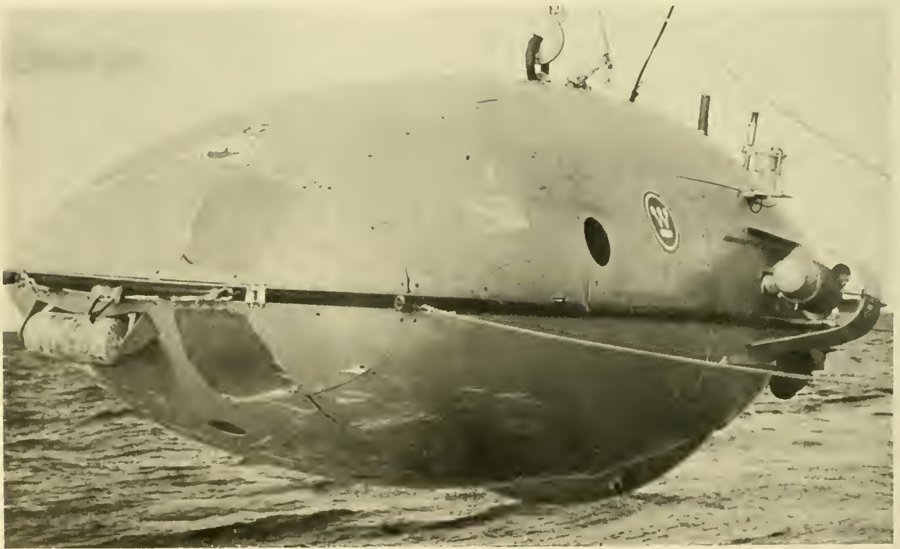
Fig 14.1 Scratches on the underside of DEEPSTAR 4000 testify to the frequency of inadvertent bottoming in submersibles (NAVOCEANO)
