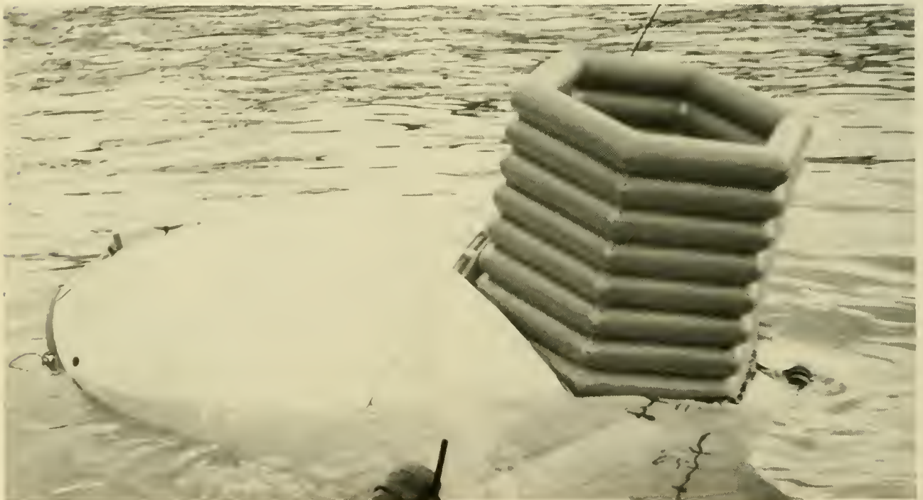
Fig. 14.15 Inflated conning tower on DEEPSTAR 4000 . (Westinghouse Corp.)
