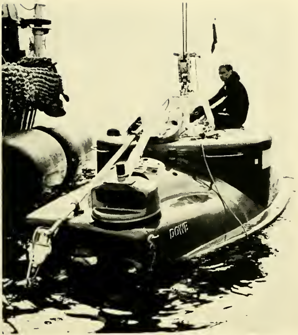
Fig. 3 24 Now a student training aid, DOWB was the only submersible to relinquish viewports in favor of fiber-optics. (Gen. Motors Inc.)
