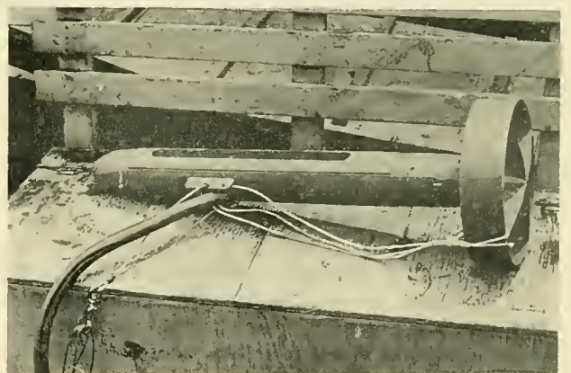
Fig. 11.7 EG & G side scan sonar recorder and transducer. (NAVOCEANO)
