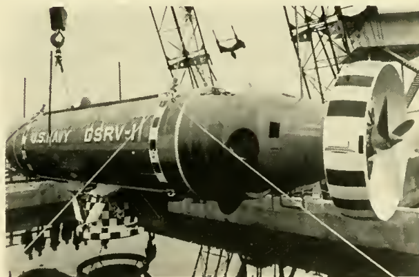
Fig. 15.3 The DSRV-1 , capable of rescuing 24 personnel from a military submarine at 3,000 feet. The black and white bell on the underside is configured to mate with the distressed submarine (U.S. Navy)
