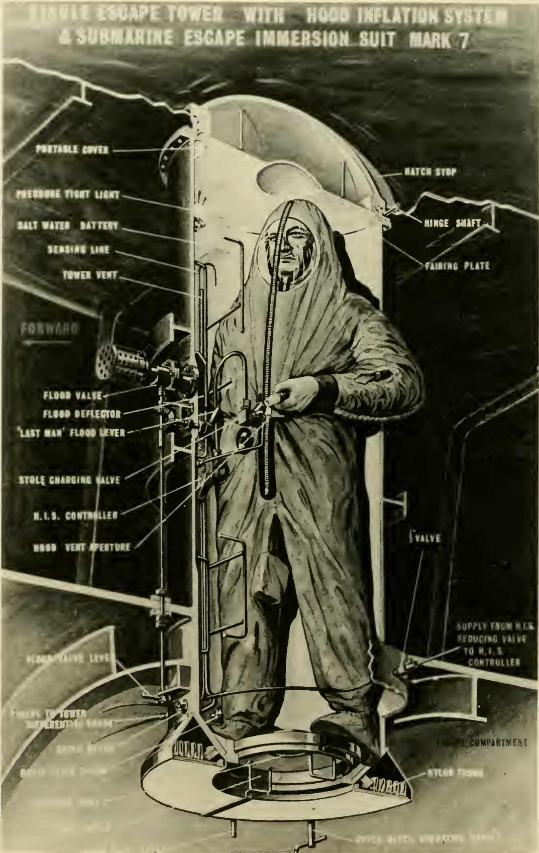
Fig 14.6 The Royal Navy's Hood Inflation System and Submarine Immersion Suit Mark 7. (K R Haigh, A.U.W.E.)
