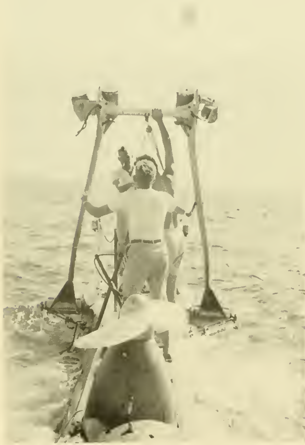
Fig. 10.8 Crewman of ALUMINAUT in the process of lowering a light boom containing four EG&G incandescent lights. (U.S. Navy)
