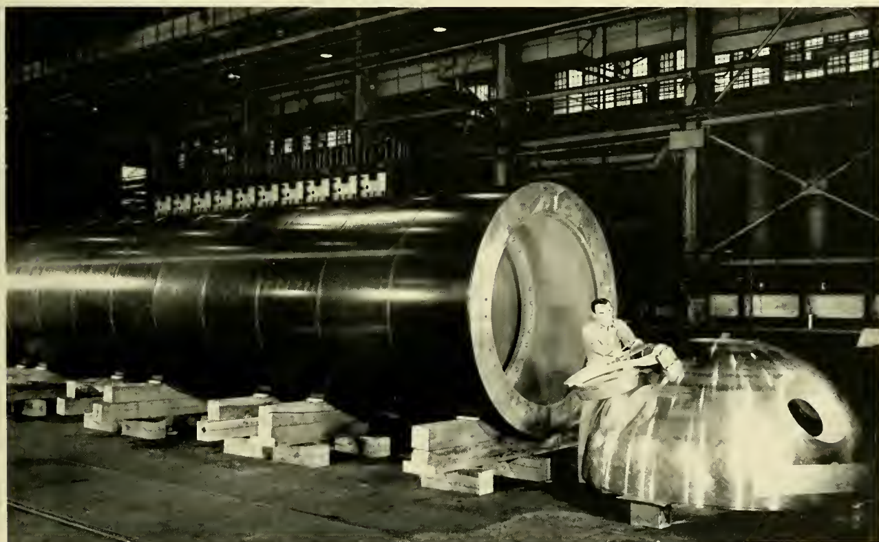
Fig. 5.7 ALUMINAUT 's pressure hull. (Reynolds Submarine Services)
