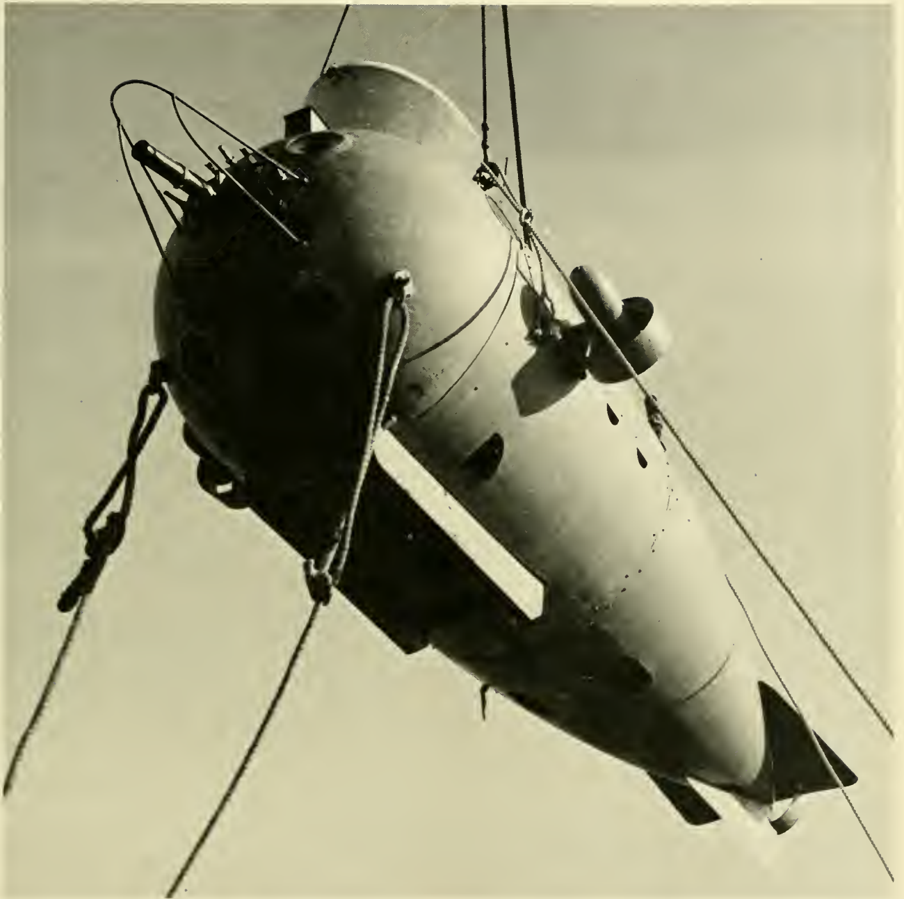
Fig 15.1 Though its bow equipment rack prohibits head-on hull collision, ASHERAH's unprotected downward-looking viewports were susceptible to contact with sharp pinnacles. (Gen Dyn./Elec. Boat)
