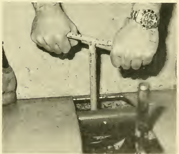
Fig. 14.4 The 200-lb lead weight (top) on SEA OTTER 's keel is manually dropped by a "T" bar wrench (bottom) from in the hull. Both ends of the weight are recessed and indexed into the keel to assure it will not rotate while being unscrewed
